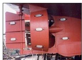
Although aluminium is also used, the most used anodes are made of Zinc, which doesn't require a tight control and delivers a continuous and efficient current.
